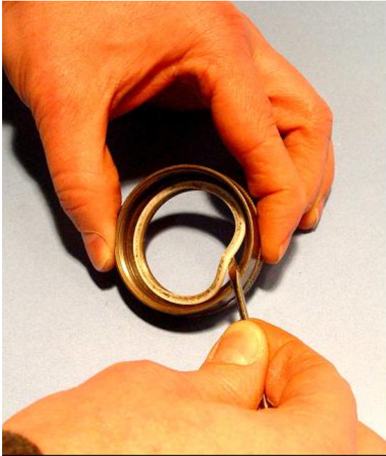
Removal of Teflon gasket from Gelman holder for high temperature applications
