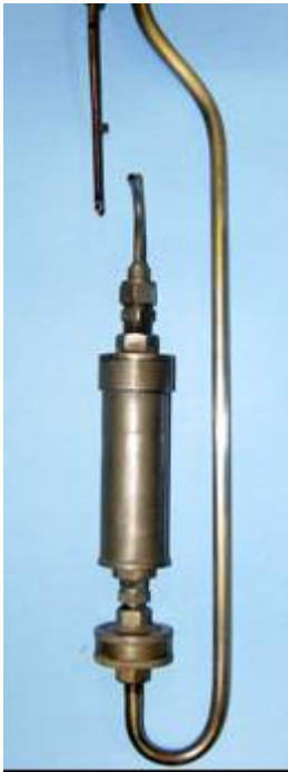
Proper orientation of nozzle relative to shephard's hook and pitot tube
