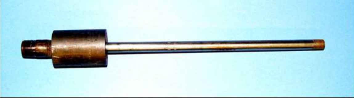
Dryer for EPA Method 17. Place between probe and filter holder to prevent condensate from draining into filter holder from the probe.
