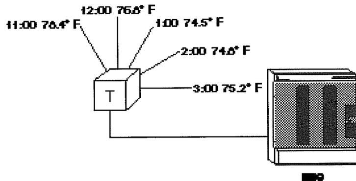
The field panel collects temperature readings from the sensor every hour.
