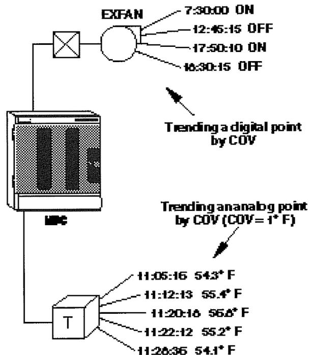
The field panel collects change of temperature information from the temperature sensor and change of state information from the fan.
