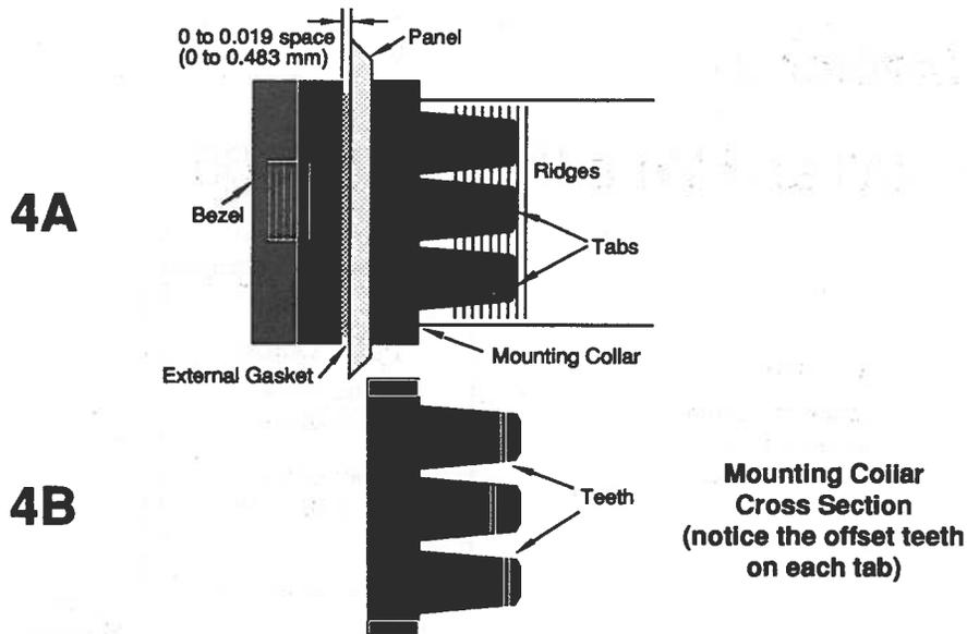
4. While pressing the front of the case firmly against the panel, slide the mounting collar over the back of the control. The tabs on the collar must line up with the mounting ridges on the case for secure installation. See Figure 4A again. Slide the collar firmly against the back of the panel getting it as tight as possible. Make sure you cannot move the case within the cutout, if you can you do not have a NEMA 4X seal.
