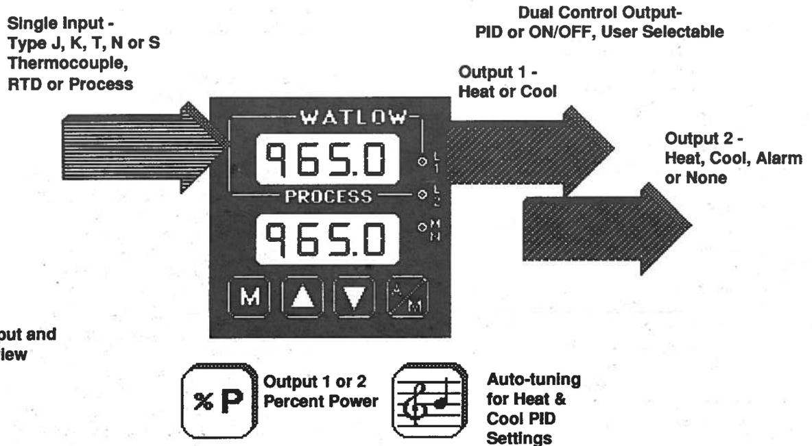
Figure 1 - Series 965 Input and Output Overview
