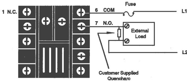
**Figure 17 - 5 Amp Mechanical Relay Wiring**
