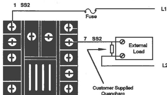
**Figure 18 - 0.5 Amp Solid State Relay Without Contact Suppression Wiring**
