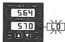
Flashing LO or HI in the lower display indicates an alarm when Ot2 = PrA or dEA. The lower display alternately shows information from the current parameter and a LO or HI alarm message at one second intervals. The alarm output is de-energized, L2 is lit.
