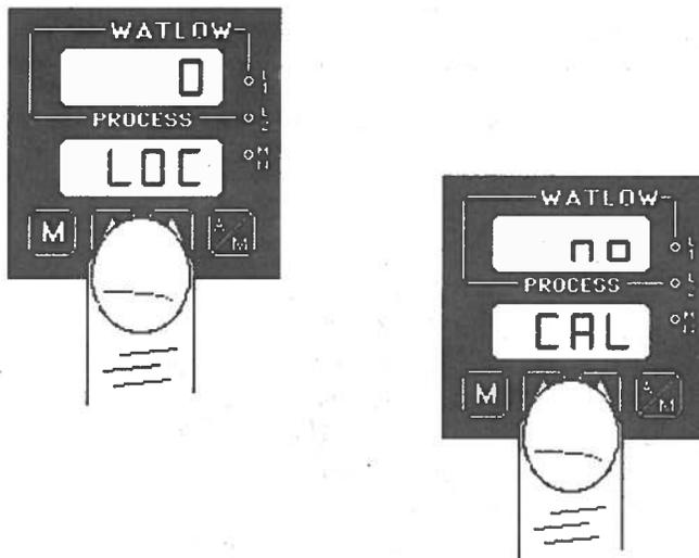
**Figure 27 - Entering the Calibration Menu.**
