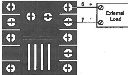
**Figure 16 - DC Output (Open Collector) Wiring**
