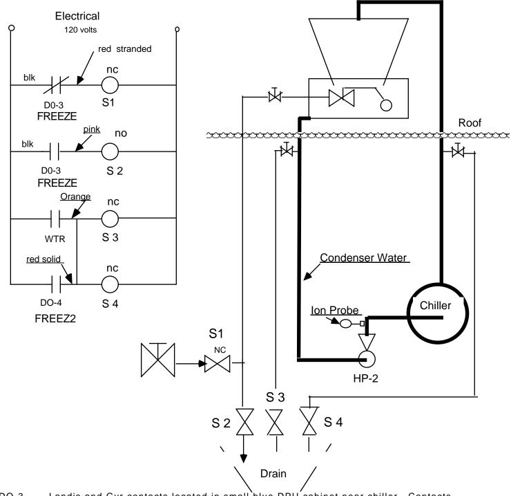
DO-3 - Landis and Gyr contacts located in small blue DPU cabinet near chiller. Contacts activate when outside air temperature drops below 40F and and deactivate when outside air temperature returns above 45F. The control point for this contactis defined as FREEZE in CPU Program 001.PGM. FREEZE point address is 00110104.
