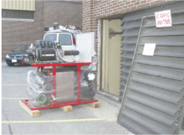
Figure 6. Multistack Turbocor Unit
